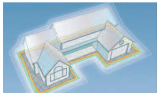
For existing buildings, the only practical method to provide protection is to treat the soil with a liquid termiticide. There are two types which are classified by their mode of action:
